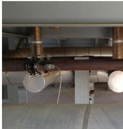
distinction. A low dB level indicated an empty pipe, and a high dB level indicated the presence of water (Figure 3).
